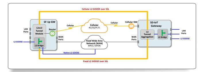
A virtual bridge in RAD's SecFlow-1p IIoT gateway receives these packets and forwards them to the SD-IoT client, which encapsulates the L2 packets over L3, encrypts them using SSL and transmits them over the cellular link (or any other WAN link available). If the SecFlow-1p is also connected to an existing fiber network (G-PON, SDH, SONET, MPLS), the packets are also forwarded to this native interface, without a L3 encapsulation for fast transmission to neighboring substations.
